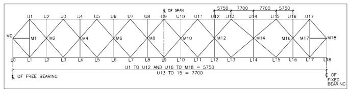
Fig. 4: Revised span configuration of the anchor span fabricated during cantilever launching
