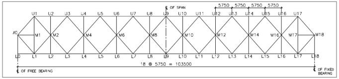
Fig. 3 : Original span configuration
