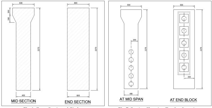
Fig 6: Cross Section of Girder
