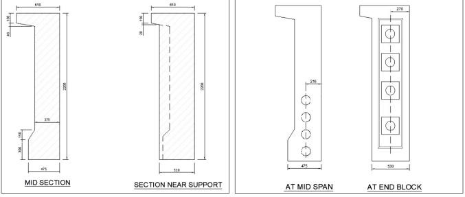
Fig 2: Cross Section of Girder
