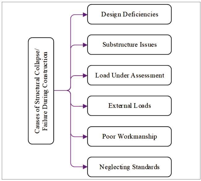
Fig. 1: Failure of structures during construction
