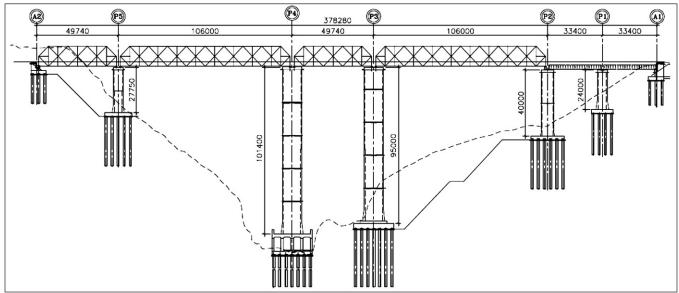
Fig. 1 : Elevation of the bridge  $\$
