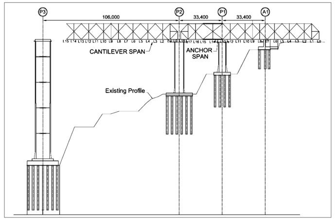
Fig. 2 : Position of cantilever span during launching
