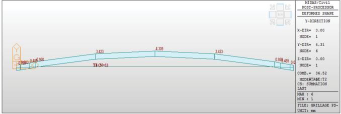
Fig. 4: Lateral Deflection of Girder as per Midas Analysis (only 4 to 5mm) lateral Bending
