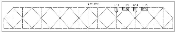
Fig. 7 : Splice at U13 and U14 joint in the original span designed for cantilever launching
