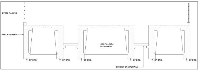
Fig 1: Cross Section of Superstructure
